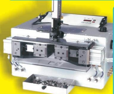
SUPERCUT/TOCF automatic machine is designed to cut and form tubed radial components type TO220, TO218, TO126.
