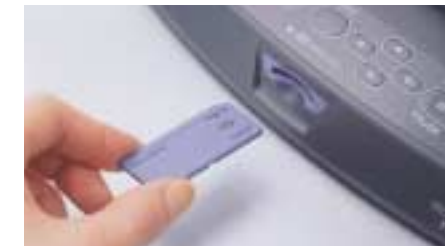
The slot can accept Memory Sticks of capacities up to 126 MB.
